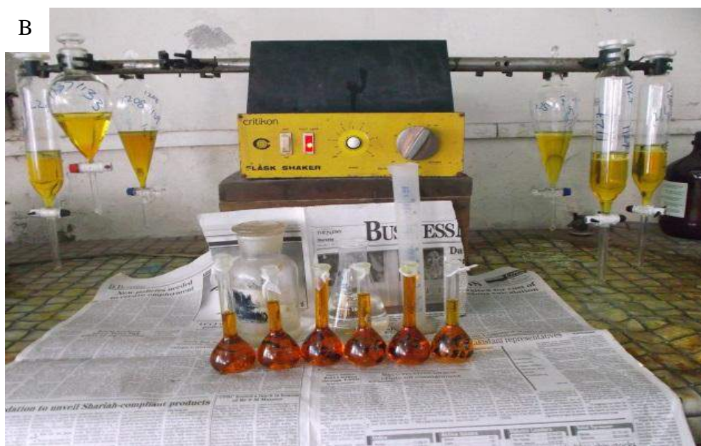
Fig. 2.5. Photographs showing preparation of stock solution for gold A: samples in pyrex beaker having aqua regia for gold digestion lying on hot plate, B: flask shaker used for the separation of gold through MIBK.
