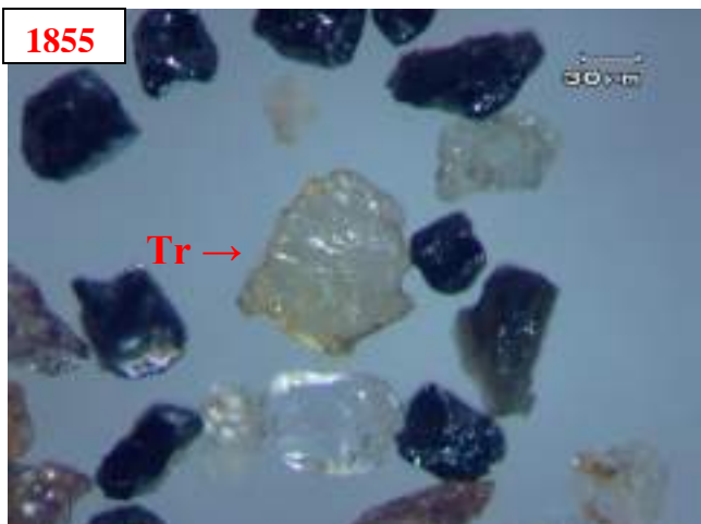
Plate 7. View of the Heavy minerals in the pan-concentrate samples from Kohat and Bannu divisions under stereomicroscope. Hem (hematite), Mag (magnetite), Fl (fluorite), Ol (olivine), Tr (tremolite).
