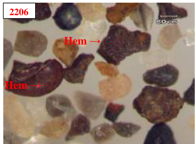
Plate 8. View of the heavy minerals in the pan-concentrate samples from D. I. Khan Division under stereomicroscope Grt (Garnet), Zrn (Zircon), Rt (Rutile), Tur (Tourmaline), Ep (Epidote), Hem (Hematite),.
