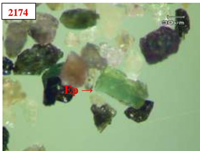
Plate 8. View of the heavy minerals in the pan-concentrate samples from D. I. Khan Division under stereomicroscope Grt (Garnet), Zrn (Zircon), Rt (Rutile), Tur (Tourmaline), Ep (Epidote), Hem (Hematite),.
