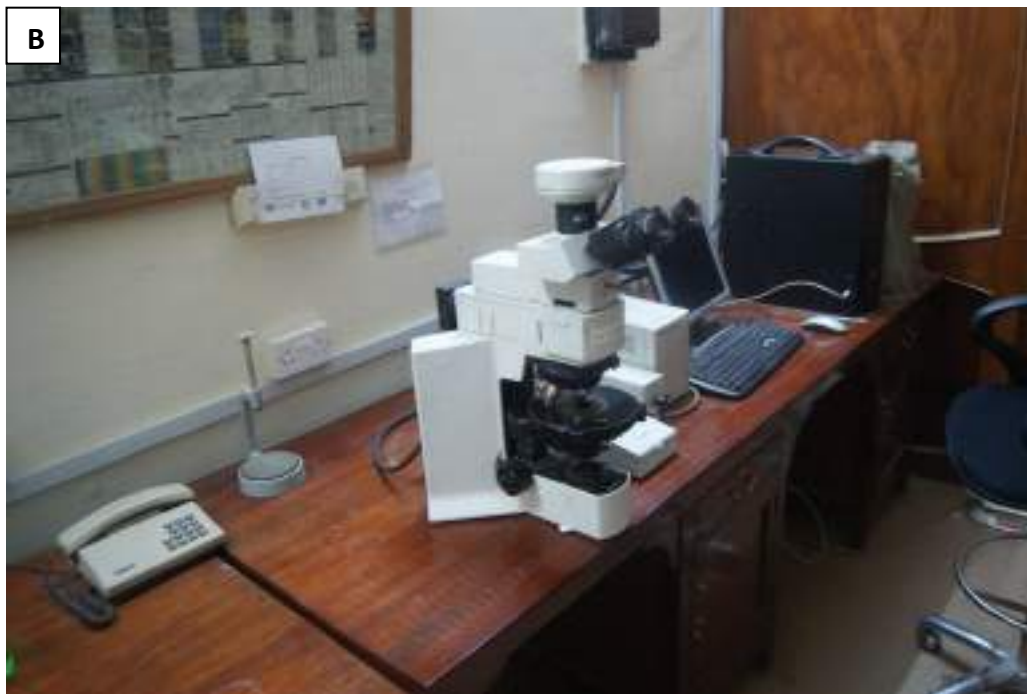
Fig. 2.3. (A): Photograph showing stereoscopic microscope used for heavy minerals mineralogical study, (B): Photograph showing polarized microscope used for petrographic studies of the rock samples.
