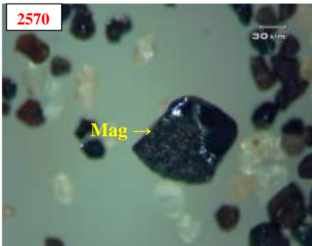
Plate9. View of the Heavy minerals in the pan-concentrate samples from D.I. Khan Division under stereomicroscope. Amp (Amphibole), Spn (Sphene), Ap (Apatite), Mnz (Monazite), Mag (Magnetite), Chl (Chlorite)
