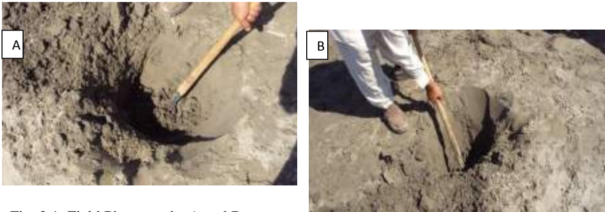
Fig. 2.1. Field Photographs A and B showing the samples collection for pan concentration.
