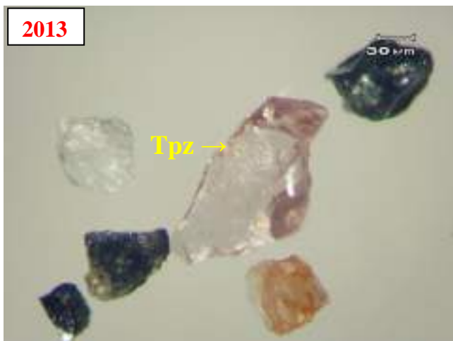
Plate 6. View of the Heavy minerals in the panned-concentrate samples from Kohat and Bannu divisions under stereomicroscope. Rt (rutile), Ap (apatite), Ep (epidote), Hbl (hornblende), Tpz (topaz), Pxn (pyroxene).
