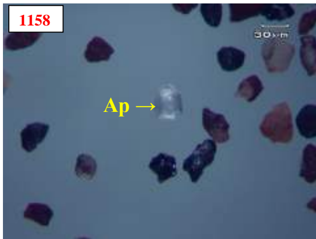
Plate4. View of the Heavy minerals in the pan-concentrate samples from Peshawar Basin under stereomicroscope. Chl (chlorite), Fl (fluorite), Ap (apatite), R.F (rock fragments).
