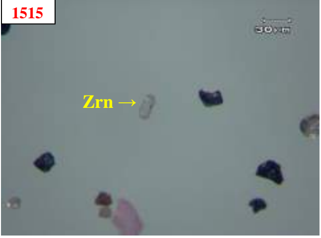
Plate 5. View of the Heavy minerals in the panned-concentrate samples from Kohat and Bannu divisions under stereomicroscope. Grt (garnet), Chl (chlorite), Tur (tourmaline), Mnz (monazite), Ilm (Ilmenite), Zrn (zircon).
